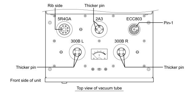
(3) After mounting all vacuum tubes, attach the vacuum tube cover.
