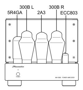
For "300B L" and "300B R", please check the sealed sticker that is on the package box and on the base.
