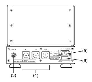
(3) Input terminal Connect an output of a pre-amplifier or attenuator.
