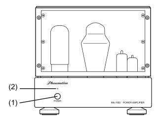
(1) POWER switch The power supply can be turned on or off by pressing the POWER switch.
