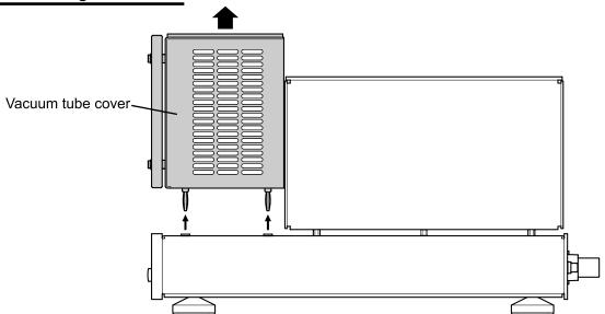
(1) Remove the vacuum tube cover straight up.
