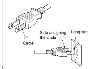
A circle is assigned on one side of the plug of the AC power cable so that better sound quality is reproduced by matching the power supply polarity with another equipment.
