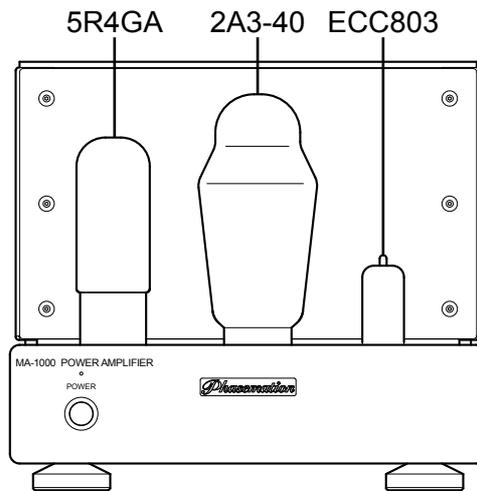
(1) The vacuum tubes are arranged in the order of "5R4GA", "2A3-40", and "ECC803" from the left.
