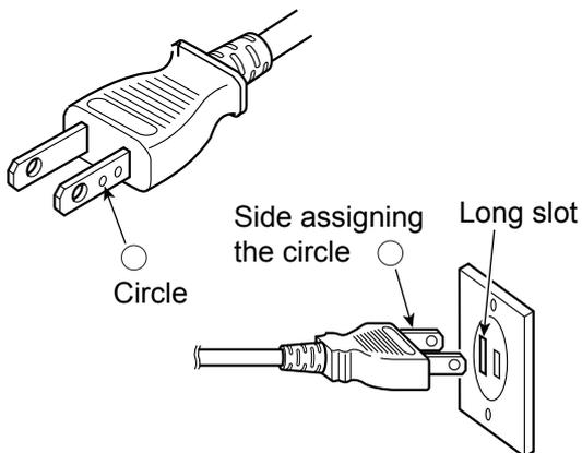
A circle is assigned on one side of the plug of the AC power cable so that better sound quality is reproduced by matching the power supply polarity with another equipment.
