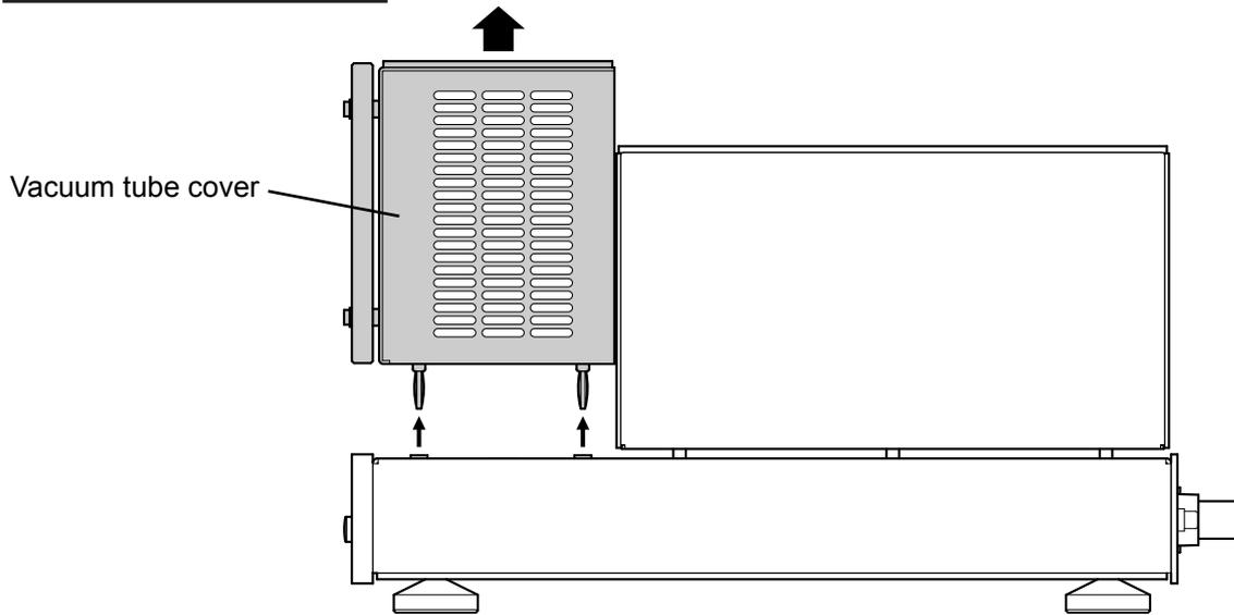
(1) Remove the vacuum tube cover straight up.
