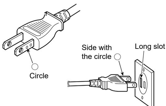
A circle is assigned on one side of the plug of the AC power cable so that better quality sound is reproduced by matching the power supply polarity with another equipment.
